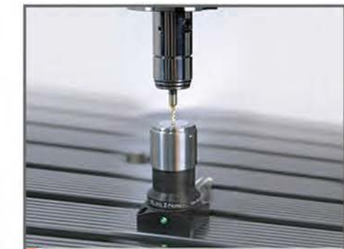
Tool breakage detector (option) Improve the efficiency of machine tools.
