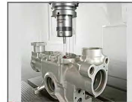
Workpiece measurement (option) Inspect parts on line, reduce defective part.
