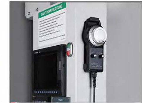
Manual pulse generator Make operation friendly.
